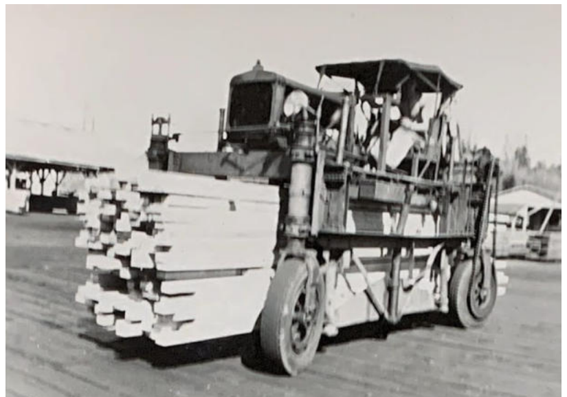
Grandpa’s photo of one of the straddle carriers he drove at the sawmill
